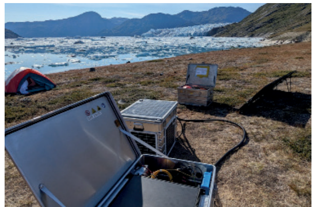
Field deployed solar powered ONYX™ in Greenland. Courtesy of Brad Lipovsky, University of Washington
